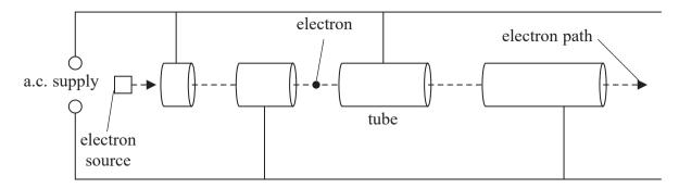
In the first part of the accelerator the drift tubes gradually increase in length, but at the end of the accelerator, the tubes are of the same length.
