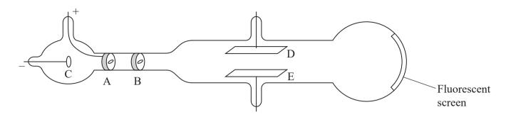
A metal disc at C emits electrons. A positively-charged disc at A accelerates the electrons along the tube. Slits in A and B produce a narrow horizontal beam of electrons. An electric field is produced between plates D and E, which can be used to deflect the beam vertically. The final position of the beam is shown on a fluorescent screen at the end of the tube.
